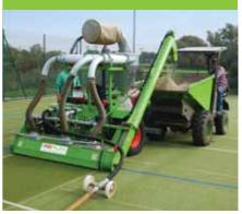
The unique REPLAY REJUVENATION® air extraction process will restore contaminated and compacted carpet to a clean 'as new' condition - extending the life of the facility at a much lower cost than replacement.
