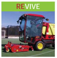
Our REPLAY REVIVE® multi-brush process penetrates the surface, decompacting and agitating the infill whilst removing dust, dirt and detritus leaving a cleaner and safer facility.
